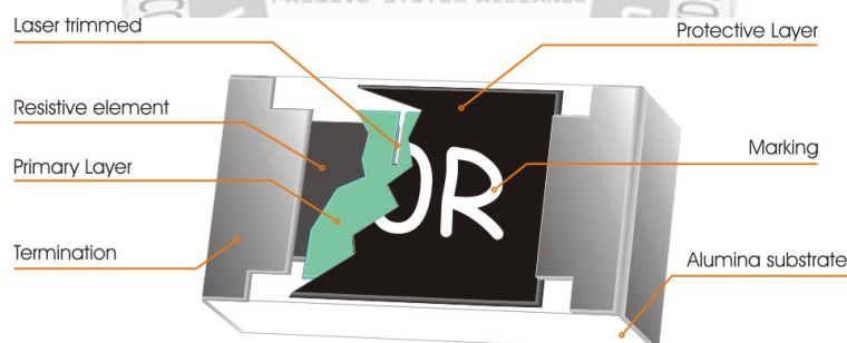
Fig 1.1. Construction of Chip-R
