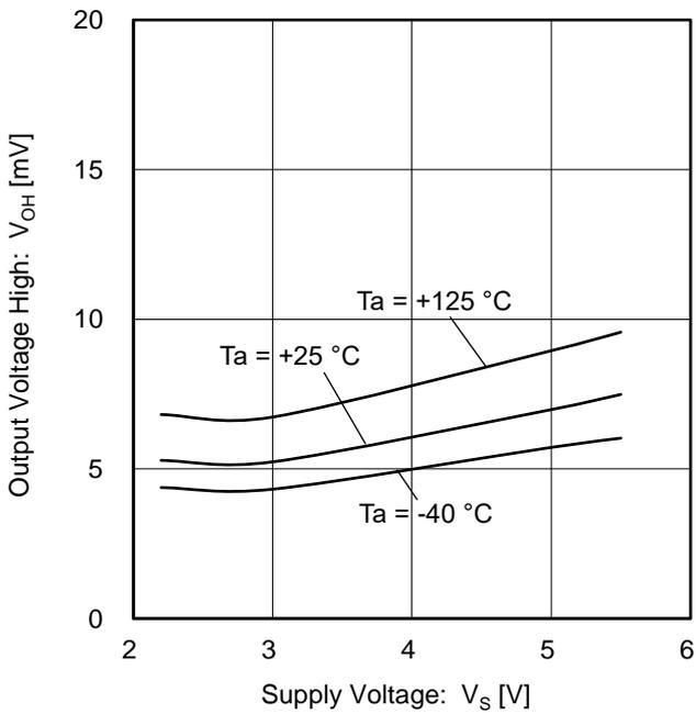
Figure 3. Output Voltage High vs Supply Voltage
