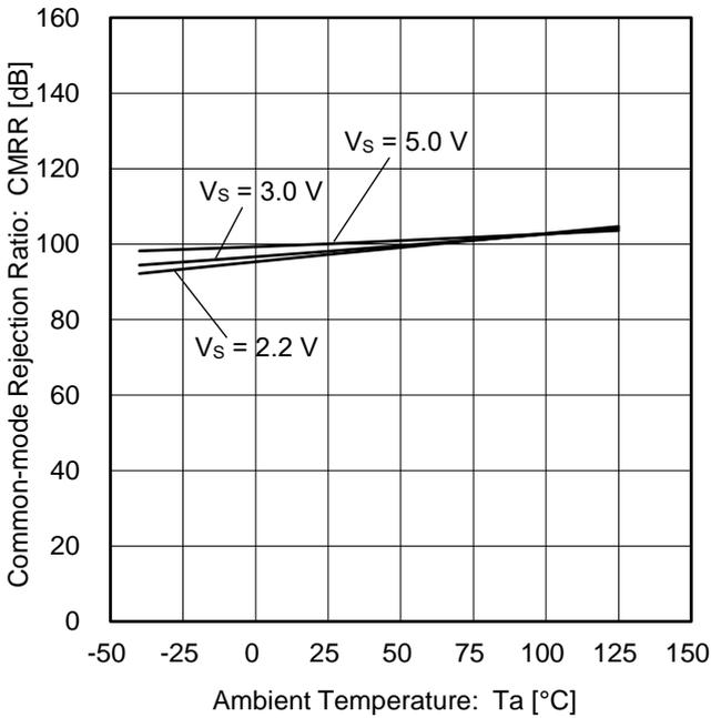
Figure 15. Common-mode Rejection Ratio vs Ambient Temperature
