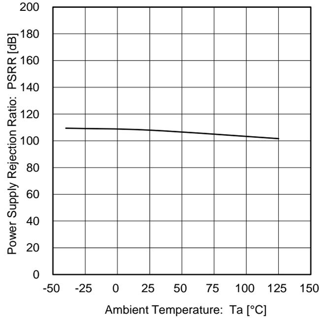
Figure 16. Power Supply Rejection Ratio vs Ambient Temperature
