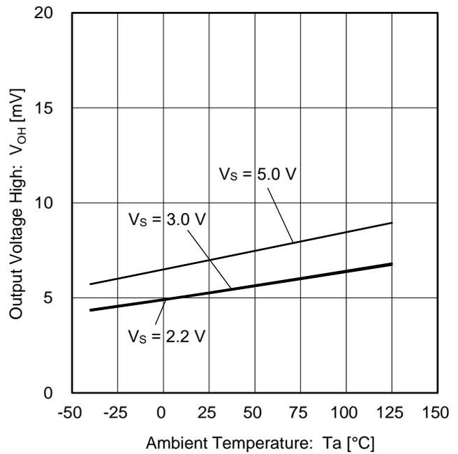
Figure 4. Output Voltage High vs Ambient Temperature
