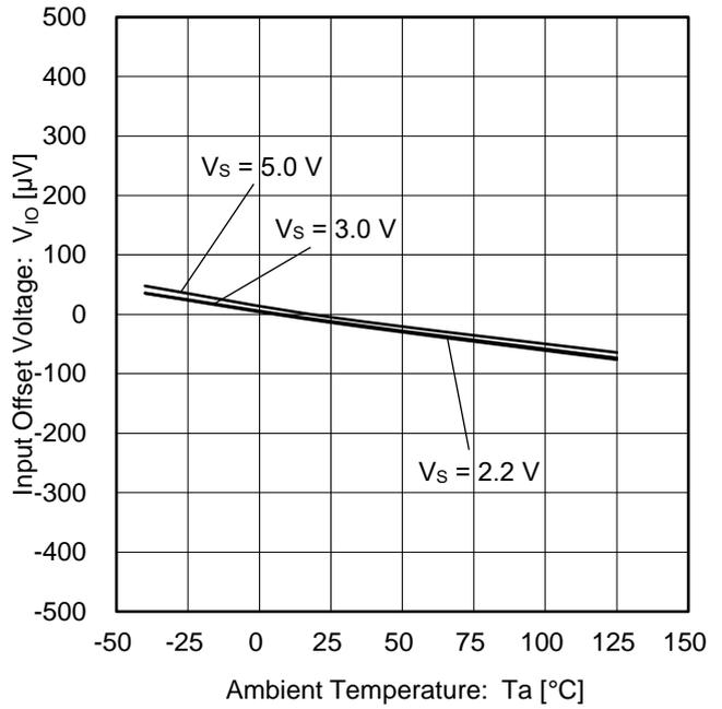
Figure 10. Input Offset Voltage vs Ambient Temperature
