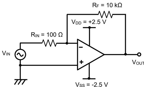
$$V_{OUT} = -\frac{R_F}{R_{IN}} V_{IN}$$
