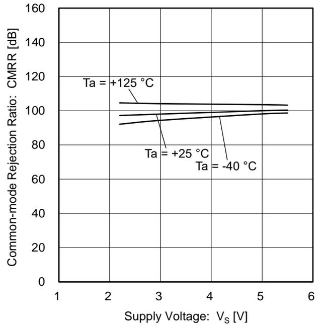
Figure 14. Common-mode Rejection Ratio vs Supply Voltage
