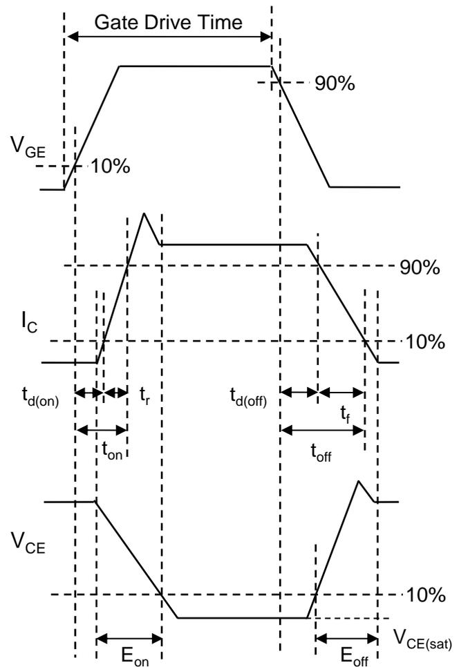
Fig.30 Inductive Load Waveform
