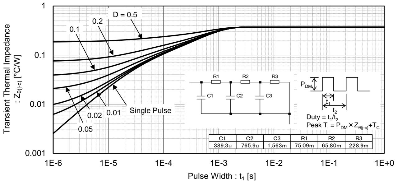
Fig.28 Typical Diode Transient Thermal Impedance
