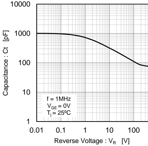
Fig.26 Typical Diode Capacitance Store Energy
