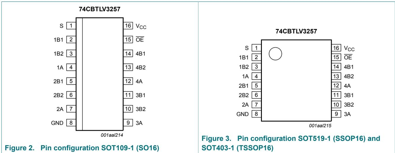
Figure 2. Pin configuration SOT109-1 (SO16)
