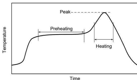
For soldering (Example : Sn/Pb )
