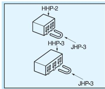
Figure 6. Terminal Jumper Description
