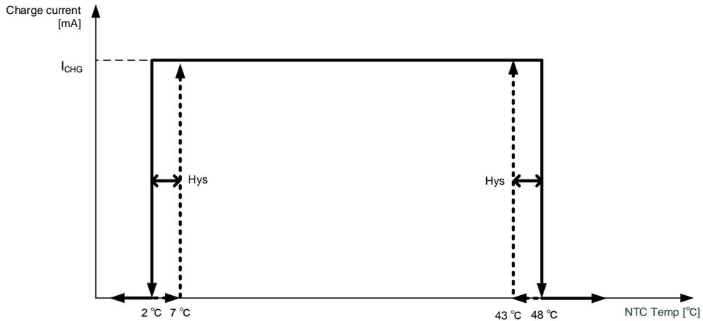
Figure 13. Charge Current vs Battery Temperature
