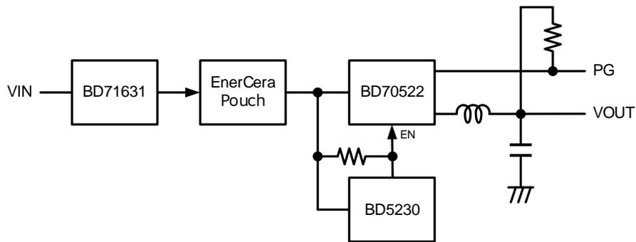
**Figure 1. Block Diagram of EnerCera and each IC**
