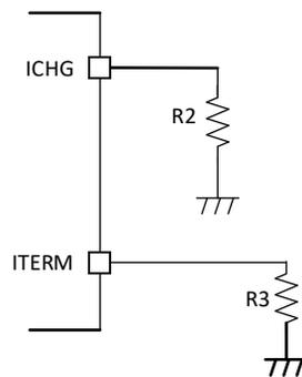
Figure 12. Resistor Setting of  $I_{CHG}$  and  $I_{TERM}$
