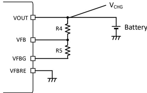
Figure 10. Resistor Setting of V<sub>CHG</sub>
