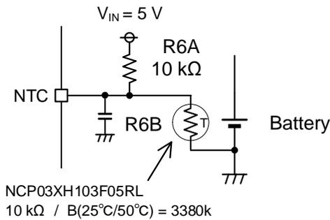
NTC terminal voltage (V<sub>NTC\_Cold</sub>, V<sub>NTC\_Hot</sub>)
