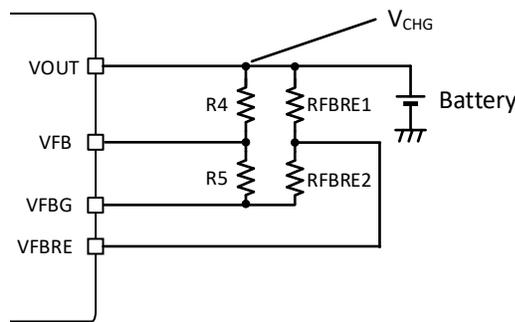
Figure 11. Resistor Setting of V<sub>RECHG</sub>
