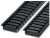
Header, Nominal current: 12 A, Rated voltage (III/2): 320 V, Number of positions: 8, Pitch: 5.08 mm, Color: black, Contact surface: Tin, Mounting: THR soldering, Two-in-one – Pin strips must always be made up of a left (L) and a right (R) segment. Please allow for the corresponding counterpart from the accessories to complete the THR pin strip.
